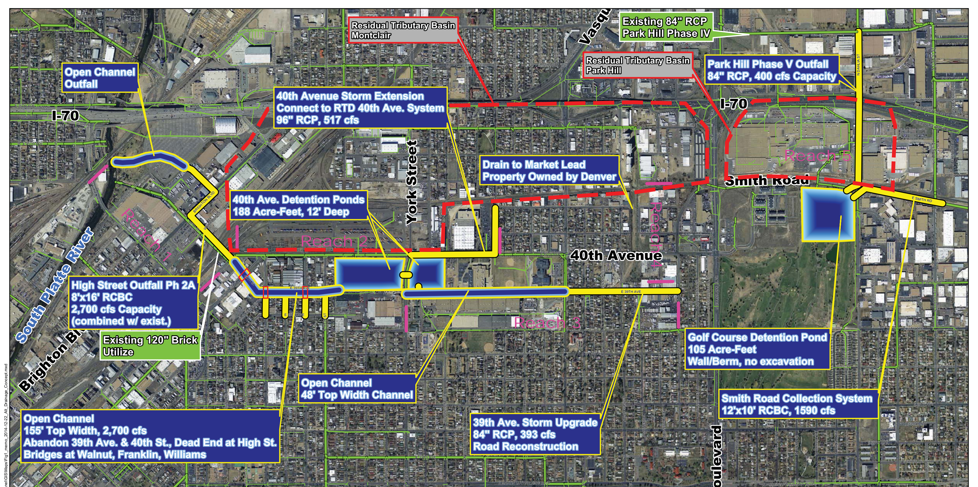
CONFIDENTIAL FIGURE 1 DRAFT CCD I-70 PCL ALTERNATIVE DRAINAGE CONCEPT PROPOSED 100-YEAR SYSTEM MONTCLAIR AND PARK HILL BASINS Technical Memorandum 2014-12-22 Detention/Conveyance/WQ Backbone Drainage System
